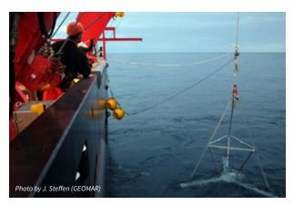
The seafloor station of the GeoSEA network, with autonomous seafloor transponders installed on 4m high tripods.
